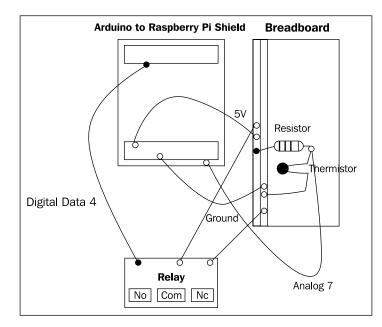
Finally, if your relay requires an external power supply, connect this. Your circuit, when connected, should look similar to the following diagram:
