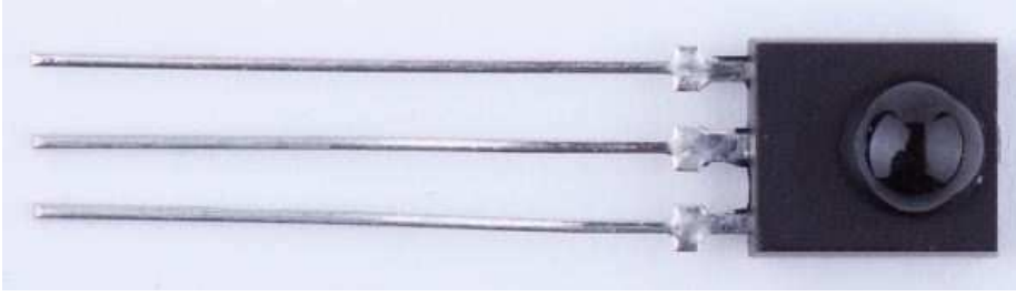
Figure 9.3: A PNA4602 infrared sensor
