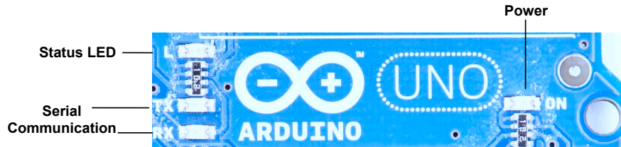
Figure 1.8: The Arduino board comes with several LEDs.
