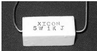
Figure 3-5: A 5-watt resistor
