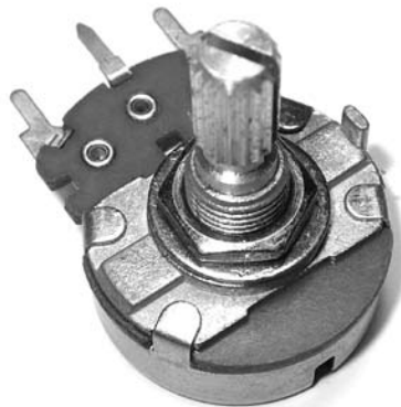
Figure 4-35: A typical linear variable resistor
