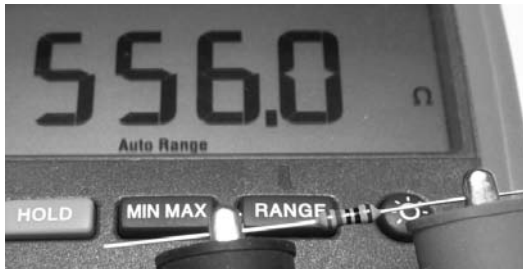
Figure 3-4: Multimeter measuring a 560-ohm 1 percent tolerance resistor
