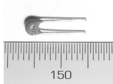
Figure 4-12: A 0.1 \mu\text{F} ceramic capacitor
