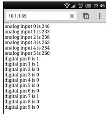
Figure 19-3: Values of the pins monitored by our station shown as a web page on any web-connected device with a web browser
