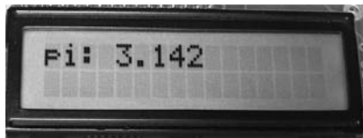
Figure 7-4: LCD displaying a floating-point number
