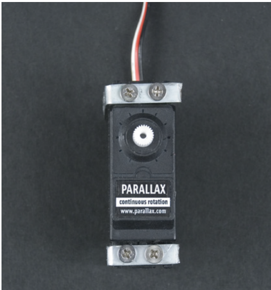
Figure 8-34. Wheel servo attachments from the front
