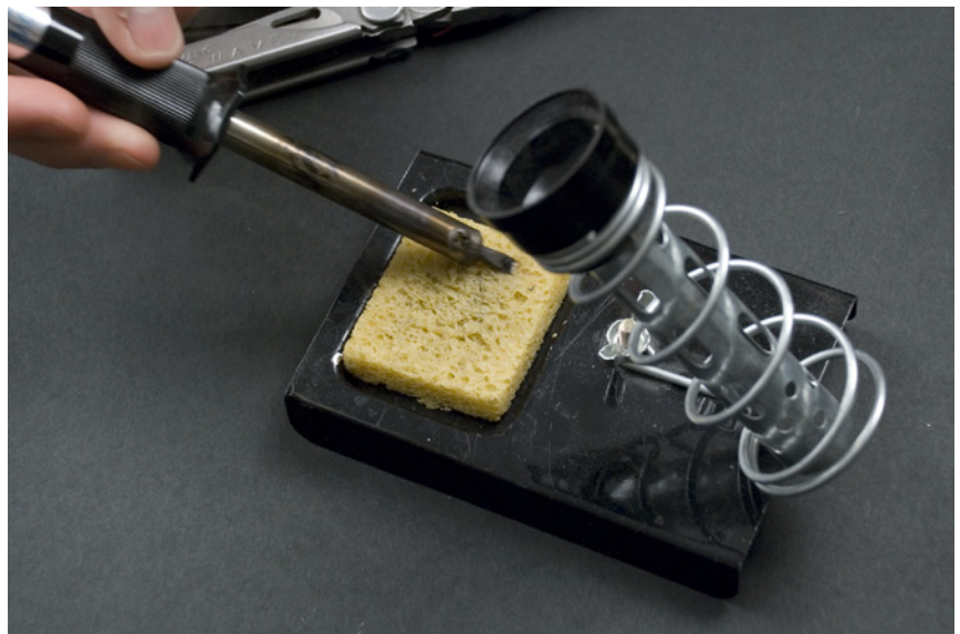
Figure 3-34. Swiping the soldering iron with a wet sponge
