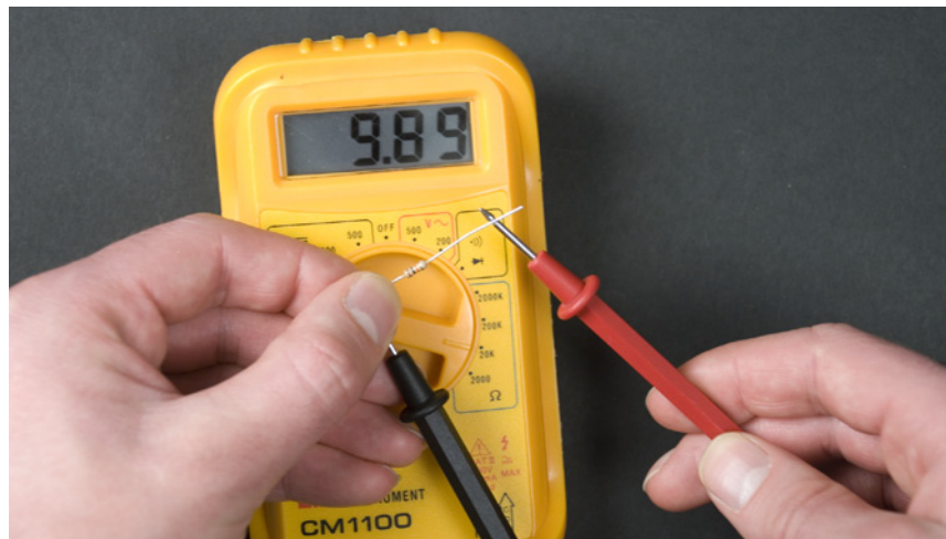
Figure 5-6. Measuring resistance with a multimeter
