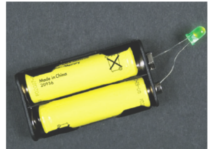
Figure 1-28. Simple closed circuit powering an LED
