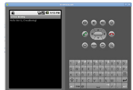
Figure 6-20. “Hello World” in the emulator, indicating a successful installation
