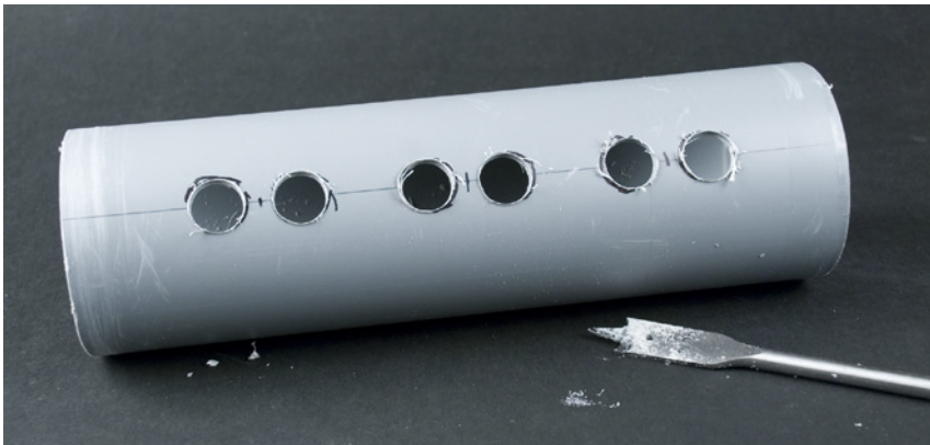
Figure 5-29. The 16mm holes for the sensors
