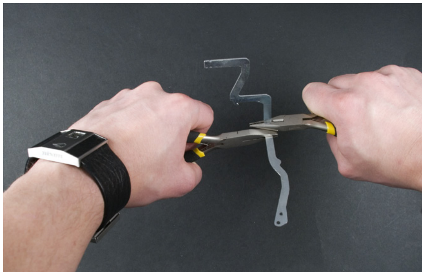
Figure 8-51. Cutting the front fork
