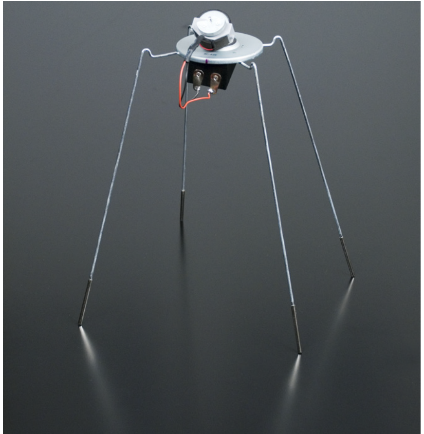
Figure 3-21. Vibrating robot, still lacking the ultrasonic sensor
