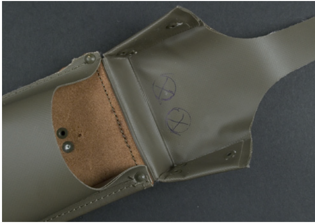
Figure 3-26. The marked positions for the ultrasonic sensor
