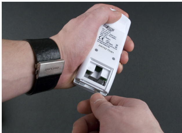
Figure 7-9. Opening with a screwdriver
