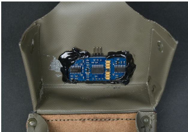
Figure 3-28. A hot-glued ultrasonic sensor
