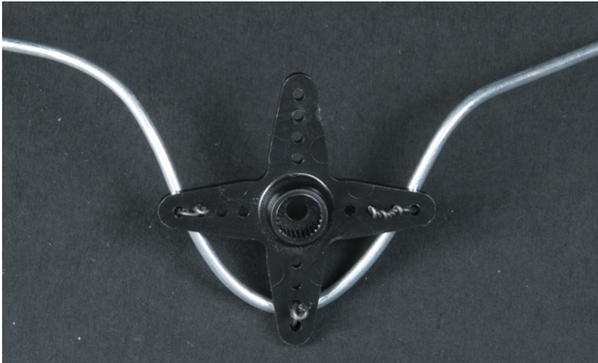
Figure 4-10. Attaching with metal wire
