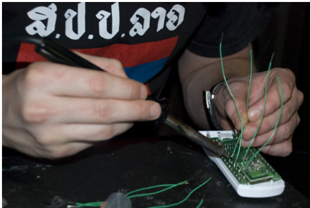
Figure 7-15. Soldering wires to the remote control switches
