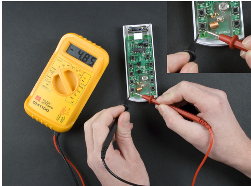
Figure 1-27. Studying a remote controller by measuring a voltage difference between two terminals of a button
