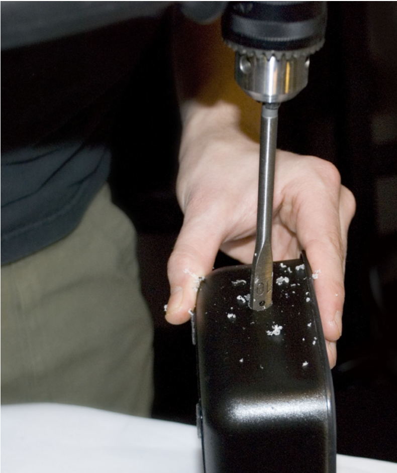
Figure 7-33. Drilling a hole for the USB cable
