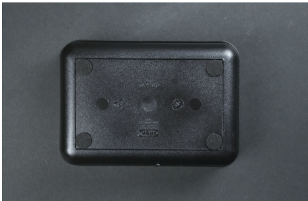
Figure 7-31. Felt pads attached to the bottom
