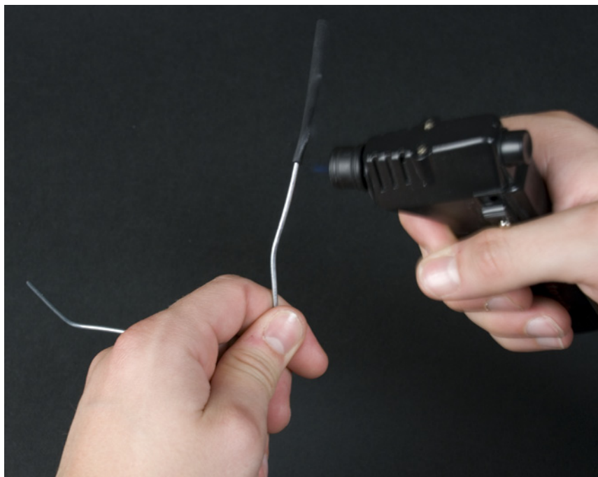
Figure 4-9. Attaching the heat-shrink tubing
