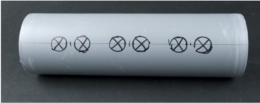
Figure 5-28. The marked ultrasonic sensor positions
