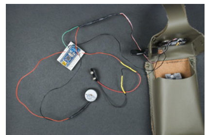
Figure 3-43. All components attached together; larger heat-shrink tubing neatly covers the individual soldered points covered by smaller heat-shrink tubing
