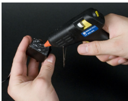
Figure 4-13. Spreading the hot glue
