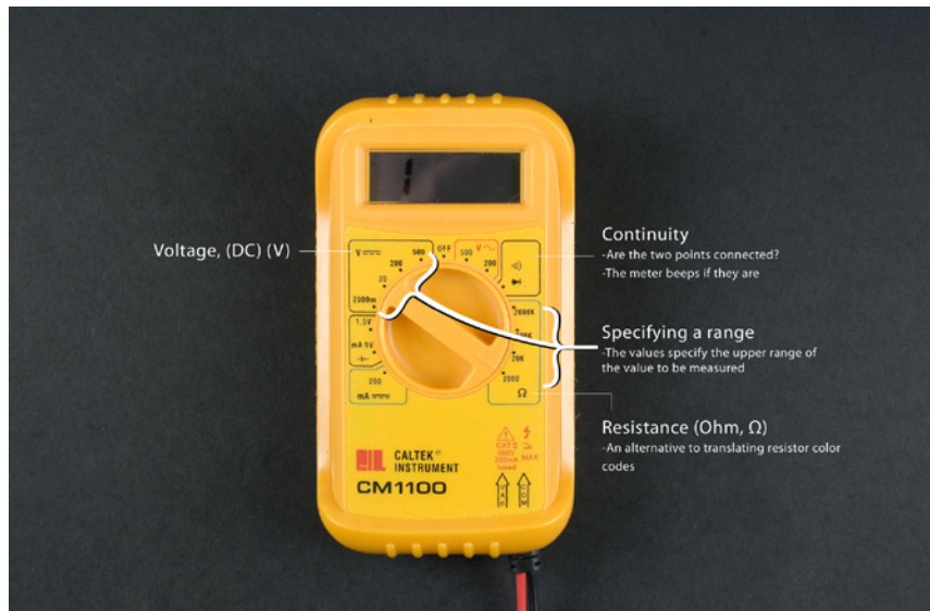
Figure 1-26. The most common functions of a multimeter
