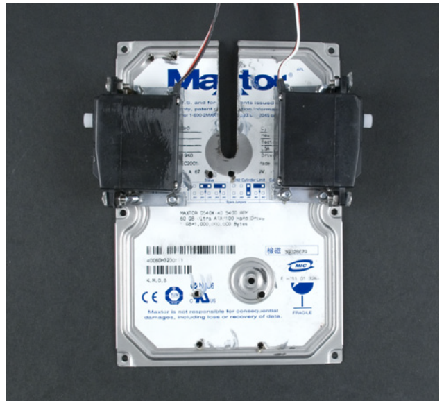
Figure 8-38. Attached wheel servos from below
