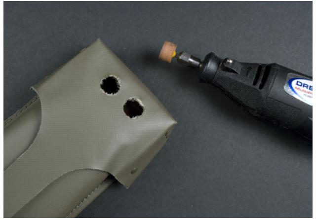
Figure 3-27. Holes created with a mini drill
