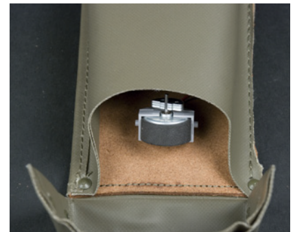
Figure 3-25. The vibration motor in place
