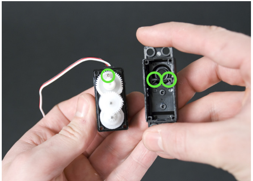
Figure 8-9. Obstructions that block rotation
