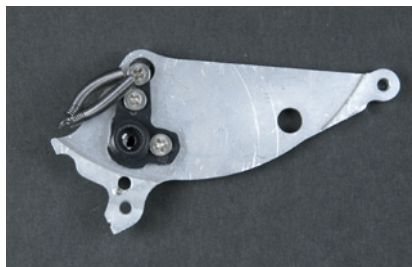
Figure 8-45. Kicker leg with servo horn attached
