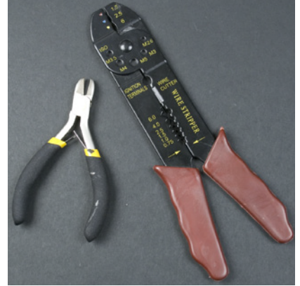
Figure 1-10. Wire stripper and side-cutter pliers are sufficient for building prototypes on a prototyping board
