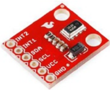
Figure 11-1. The MPL3115A2 on a Sparkfun breakout board
