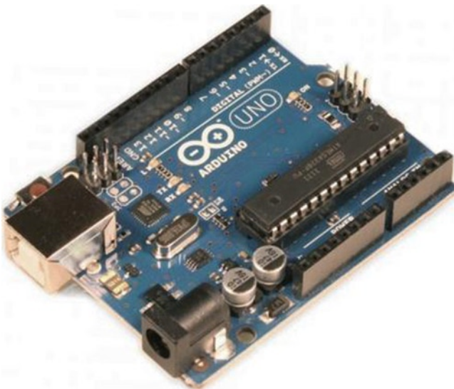
Figure 1-4. An Arduino Uno (Image courtesy of Earthshine Electronics)
