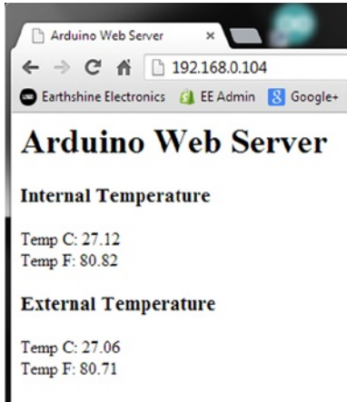
Figure 17-2. The web browser output from the Arduino web server
