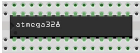
Figure 2-3. An integrated circuit (or chip) plugged across the gap in a breadboard
