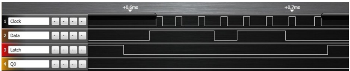
Figure 6-3. The output from the 595 shown in a logic analyzer
