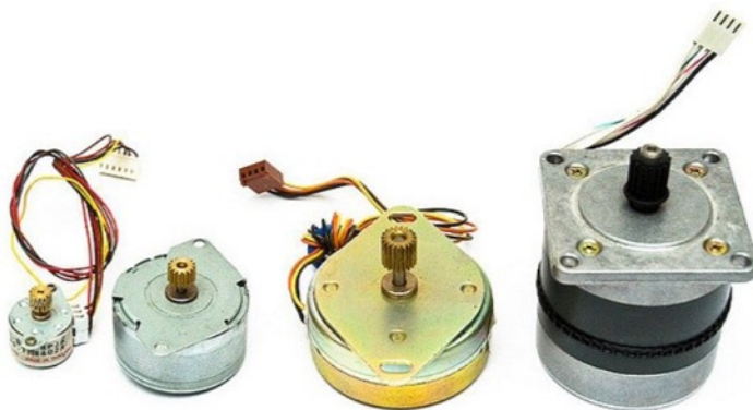
Figure 10-3. Different kinds of stepper motors (image by Aki Korhonen)
