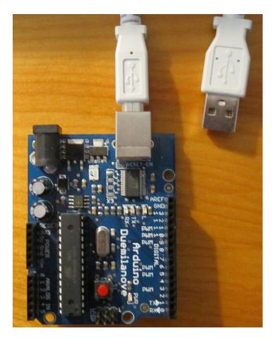
Figure 1-6. The µc board with USB cable attached.
