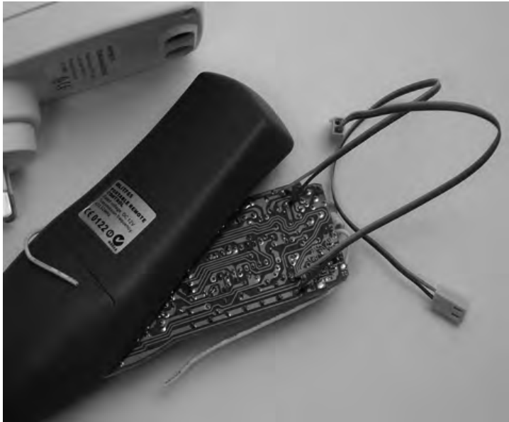
Figure 2-11. Remote control transmitter with connections in place
