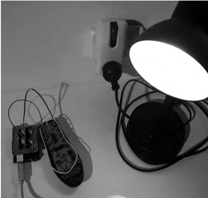
Figure 2-14. Arduino and shield using an appliance remote control to activate a lamp
