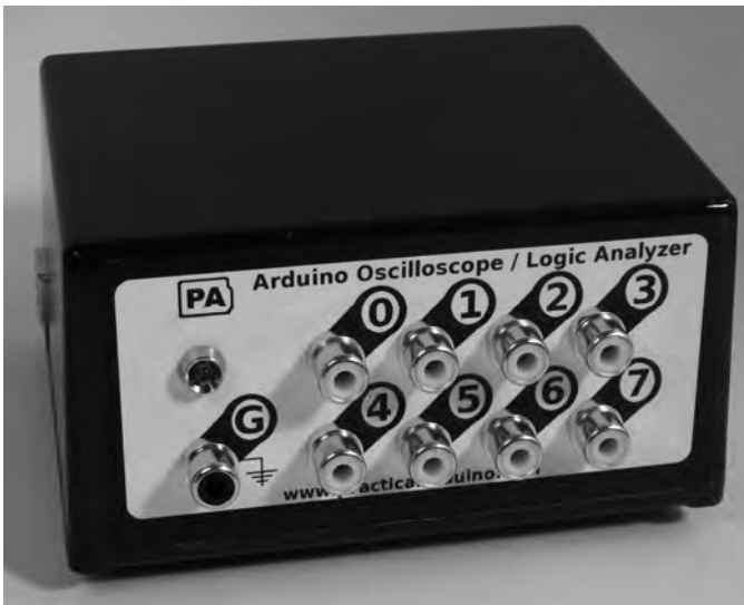
Figure 11-6. Connectors and LED mounted in front panel
