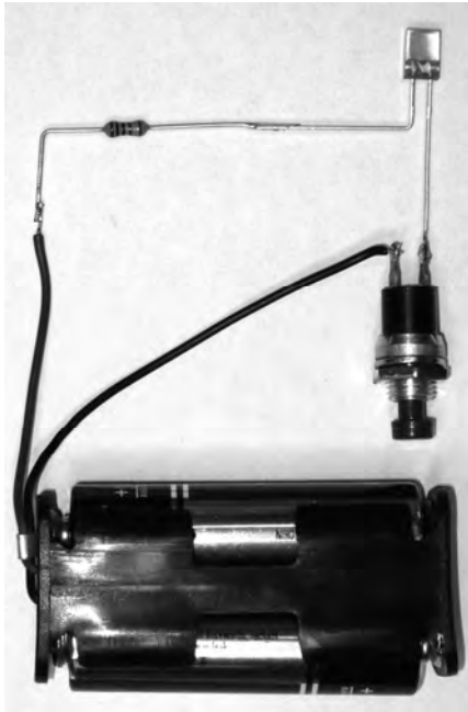
Figure 1-1. A battery, resistor, LED and switch – the hardware version of “hello world!”
