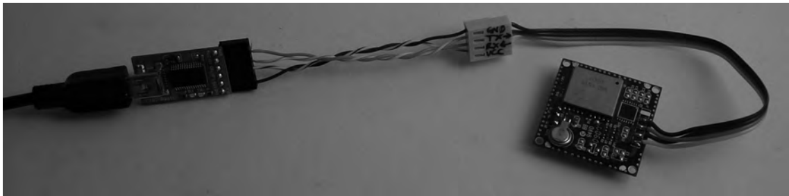
Figure 15-15. The LS20031 GPS module connected to a host computer using an FTDI adapter
