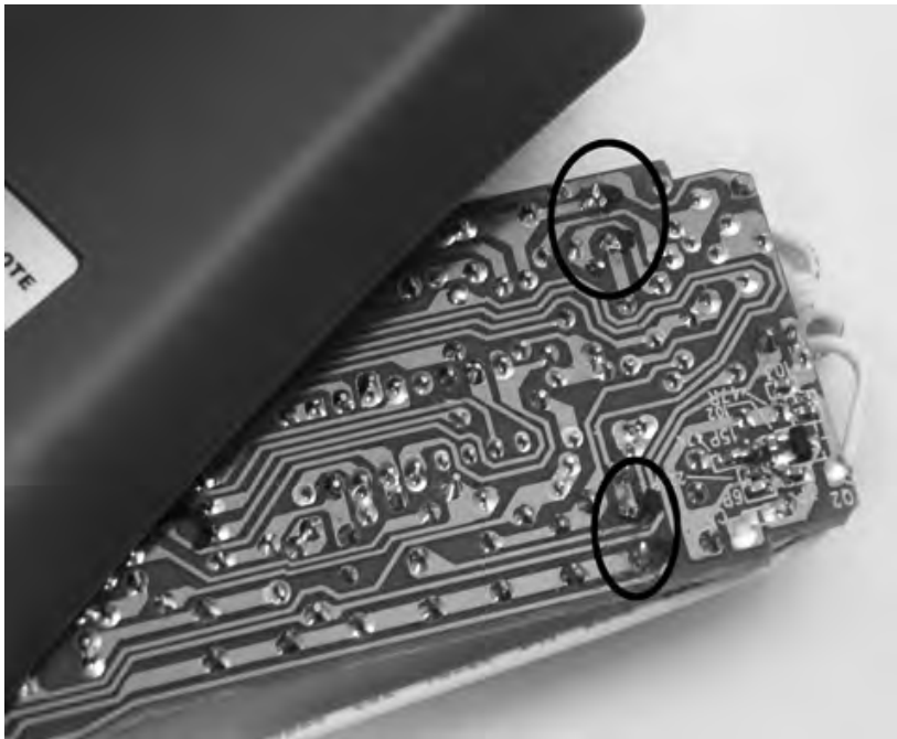
Figure 2-4. PCB of appliance remote control transmitter
