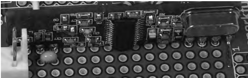
Figure 13-8. RXB1 receiver mounted on shield
