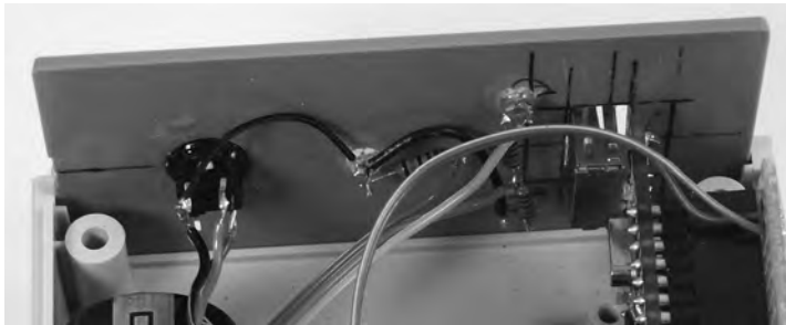
Figure 15-31. The Logging button and status LEDs glued into the front panel
